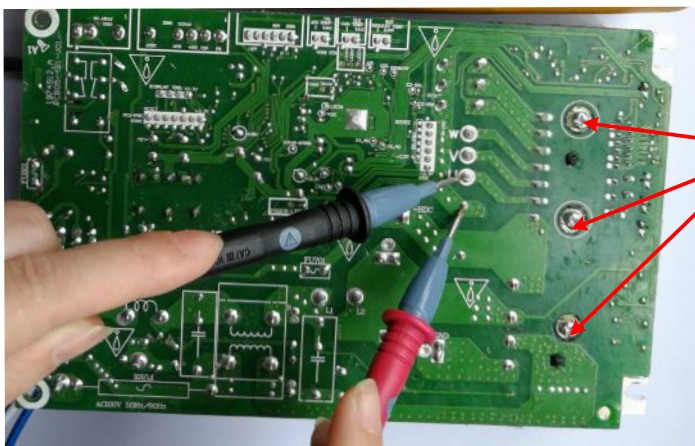
Fasten the IPM screw A
