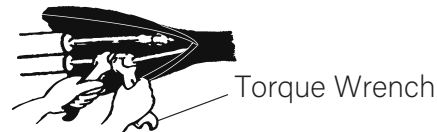
TIGHTENING TORQUE FOR PROTECTION CAPS AND FLANGE CONNECTION
